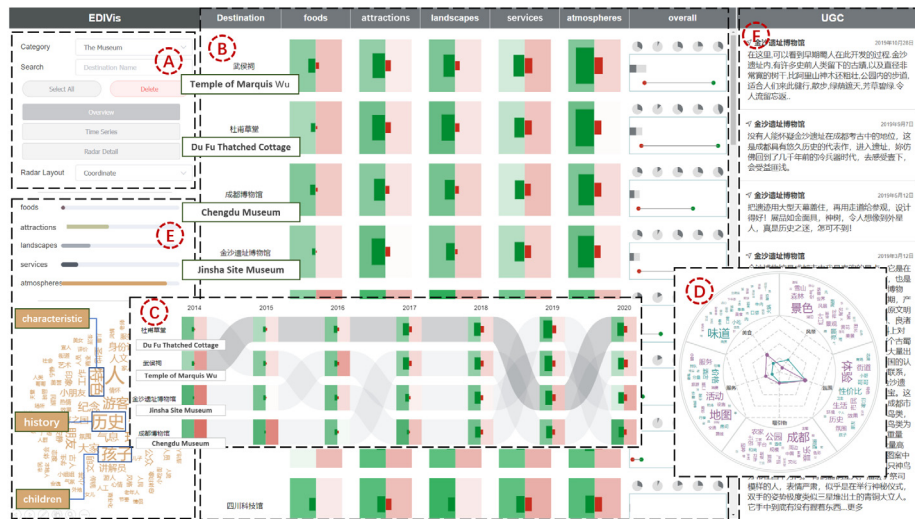
Fig. 1. MDIVis allows users to investigate and compare multiple destination images on UGC from multiple aspects. Setting panel (A) helps users to roughly filter destinations of interest, the Sentiment Matrix View (B) presents an overview of images of multiple candidate destinations, the Timing View (C) describes changes in the ranking of several destinations over the years, the Keywords Radar View (D) provides detailed information to explore and compare the destination images, and the Auxiliary View (E, F) offer extra information for users.
