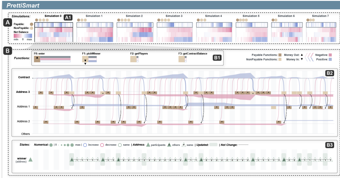
Fig. 1: The interface of PrettiSmart consists of a Simulation Overview Module (A) to provide a visual summary for each simulation (A1) generated by our simulator and a Simulation Detail Module (B) to show the details of each simulation, including the Function Summary (B1), the Function Call Details involving cryptocurrency flows and net balance changes (B2), and State Variable Changes (B3). In this figure, PrettiSmart provides a visual interpretation of a gambling smart contract, called “Lottery”, and helps investors intuitively understand the contract’s behavior after each investment and how it selects and repays the winner.
